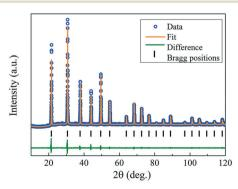
Fig. 9 Rietveld refinement results of XRD data measured on the powders obtained from the crushed as-grown GdB<sub>6</sub> single crystals.
