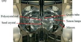
Fig. 2 (a) Schematic diagram and (b) photograph of the optical floating zone growth furnace.
