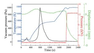
Fig. 4 Preparation process of polycrystalline GdB<sub>6</sub> by the SPS method.
