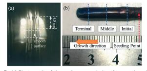
Fig. 7 (a) Photograph of the molten zone during the growth and (b) morphology of the as-grown GdB<sub>6</sub> single crystal. The growth direction and the seeding point are presented. The blue dotted lines indicate the parts for the SEM and ICP measurements.
