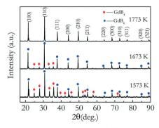
Fig. 5 XRD patterns of polycrystalline  $\mathsf{GdB}_6$  at different sintering temperatures.
