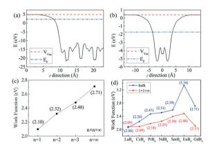
Fig. 11 Calculated electrostatic potential energy of the (100) surface of (a) bulk and (b) nanowire GdB<sub>6</sub>. Work function of bulk and  $n \times n \times \infty$  (n = 1, 2, and 3) nanowires of (c) GdB<sub>6</sub> and (d) rare earth hexaborides.
