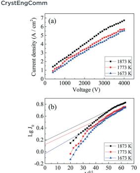
Fig. 10 (a) Thermionic emission properties and (b) Schottky curves of the  $GdB_6$  cathode at different temperatures.
