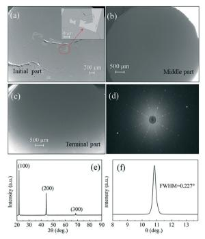
Fig. 8 (a)-(c) SEM images of the initial part, middle part and terminal part, (d) X-ray Laue diffraction photograph, (e) XRD patterns and (f) X-ray rocking curves of the GdB<sub>6</sub> single crystal.
