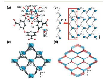
Fig. 1 (a) Coordination environment of the Zn(II) center in CP 1. Color code: Sky blue – Zn; red – O; gray – C. (b) The 1D infinite chain and 2D layered structure formed by the Zn(II) atoms and  $L^{5-}$  ligands in CP 1. (c) Perspective view of the 3D open framework in the b direction. (d) The topological network with the point symbol ( $6^6$ ).
