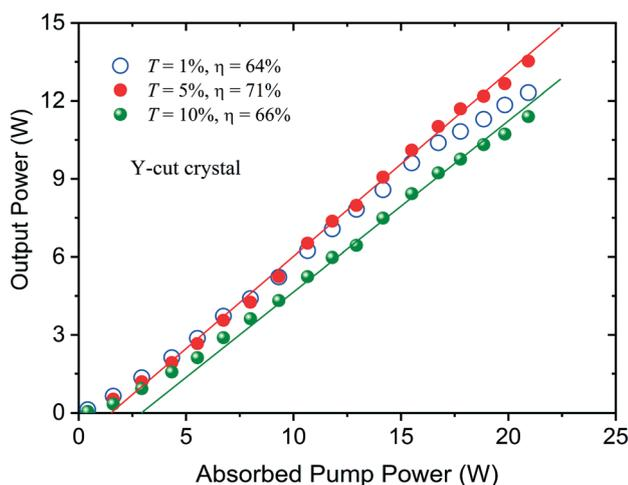
**Fig. 8** Output power versus absorbed pump power for  $T = 1\%$ ,  $5\%$ , and  $10\%$ , produced in laser operation achieved with the Y-cut crystal.
