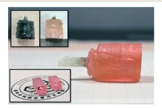
Fig. 1 Photographs of the grown Er:Lu<sub>2</sub>O<sub>3</sub> crystal boule. The inserts, in the upper left corner, show the Er:Lu<sub>2</sub>O<sub>3</sub> boule before (left) and after (right) post-growth annealing. The insert, in the lower left corner, shows the photograph of end polished rods of the grown Er:Lu<sub>2</sub>O<sub>3</sub> crystal.
