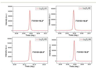
Fig. 4 Rocking curves of the Er:Lu<sub>2</sub>O<sub>3</sub> crystal.
