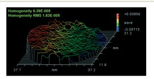
Fig. 6 Optical homogeneity in realistic fixed 3D views of the Er:Lu<sub>2</sub>O<sub>3</sub> single crystal, which shows the wavefront variations in 3D views. The unit of the 3D views of the measurement results is wavelength ( $\lambda$  = 632.8 nm), representing the relative change of the refractive index at different positions.
