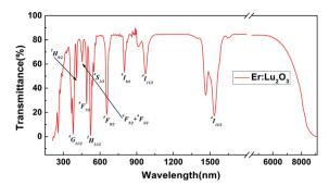
Fig. 7 Transmittance spectrum of the 2.1 mm thick uncoated  $\rm Er: Lu_2O_3$  single crystal sample.
