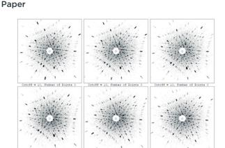
Fig. 5 Characteristic Laue back-reflection patterns at different positions.
