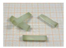
Fig. 2  $Lu_2O_3$  crystal seeds with the <541> direction obtained by the HEM.
