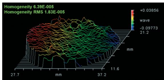
Fig. 6 Optical homogeneity in realistic fixed 3D views of the Er:Lu<sub>2</sub>O<sub>3</sub> single crystal, which shows the wavefront variations in 3D views. The unit of the 3D views of the measurement results is wavelength ( $\lambda = 632.8$  nm), representing the relative change of the refractive index at different positions.
