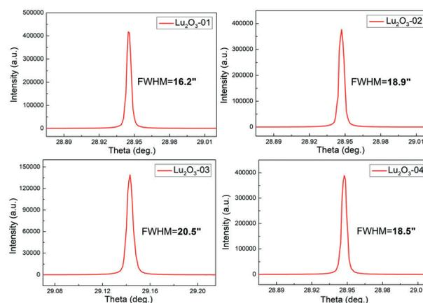
Fig. 4 Rocking curves of the  $\text{Er}:\text{Lu}_2\text{O}_3$  crystal.
