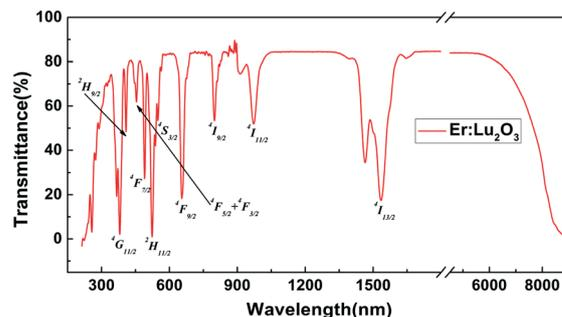
Fig. 7 Transmittance spectrum of the 2.1 mm thick uncoated Er:Lu<sub>2</sub>O<sub>3</sub> single crystal sample.
