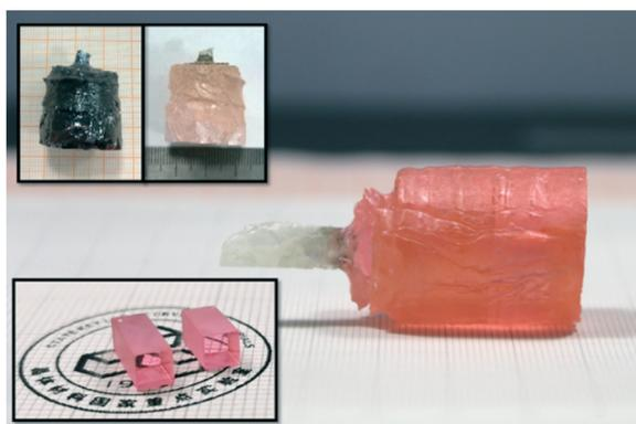
**Fig. 1** Photographs of the grown  $\text{Er}:\text{Lu}_2\text{O}_3$  crystal boule. The inserts, in the upper left corner, show the  $\text{Er}:\text{Lu}_2\text{O}_3$  boule before (left) and after (right) post-growth annealing. The insert, in the lower left corner, shows the photograph of end polished rods of the grown  $\text{Er}:\text{Lu}_2\text{O}_3$  crystal.
