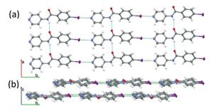
Fig. 3 INPBA structure: (a) 2D sheets formed by  $N_{pyr}{\cdot\cdot\cdot\cdot}I$  halogen bonding in green and perpendicular N-H···O=C carboxamide hydrogen bonds in blue; (b) isolated layers. Thermal ellipsoids are drawn at the 50% probability level.
