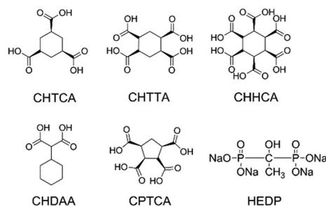
**Fig. 1** Structures of key cyclic polycarboxylic acids and the common phosphorus based inhibitor, HEDP. Compounds shown are: (1 $\alpha$ ,3 $\alpha$ ,5 $\alpha$ )-1,3,5,-cyclohexanetricarboxylic acid (CHTCA); cyclohexane-1,2,4,5-tetracarboxylic acid (CHTTCA); 1,2,3,4,5,6-cyclohexanehexacarboxylic acid (CHHCA); 1,1-cyclohexandiacetic acid (CHDAA); *cis,cis,cis,cis*-1,2,3,4-cyclopentanetetracarboxylic acid (CPTCA); tetra sodium salt of hydroxyethane 1,1-diphosphonic acid (HEDP).
