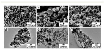
Fig. 3 SEM and TEM images of the hierarchically porous HKUST-1\_At samples produced at different synthesis times: (a and d) HKUST-1\_A1; (b and e) HKUST-1\_A10; (c and f) HKUST-1\_A30.
