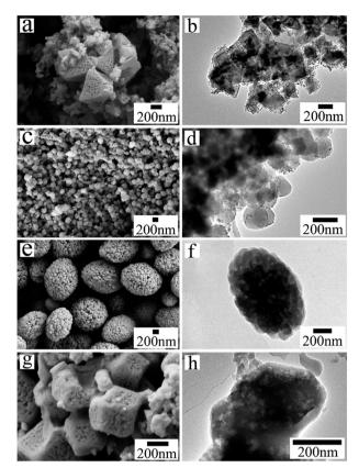
**Fig. 2** SEM and TEM images of the hierarchically porous MOFs: (a and b) HKUST-1\_A1; (c and d) ZIF-8\_A1; (e and f) ZIF-61\_A1; (g and h) ZIF-90\_A1.
