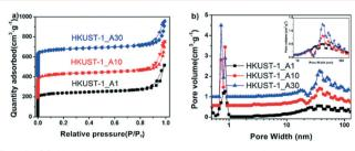
Fig. 4 (a) N<sub>2</sub> adsorption-desorption isotherms of the hierarchically porous HKUST-1\_At (t = 1, 10, 30) samples. For clarity, isotherms of the HKUST-1\_A10 and HKUST-1\_A30 samples are offset by -190 and  $-400~{
