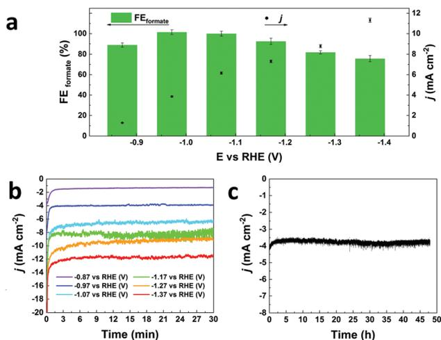
Fig. 4 (a) Faradaic efficiency (FE, green bars) and current density ( $j$ , black dots) in the reduction of  $\text{CO}_2$  to formate with BiSub@AC-400 as electrocatalyst in  $\text{CO}_2$ -saturated 0.5 M  $\text{NaHCO}_3$  at the indicated potentials; (b) the corresponding chronoamperometric study at various potentials; (c) 48 h chronoamperometry at  $E = -0.97$  V vs. RHE.
