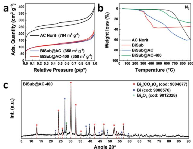
Fig. 3 (a) N<sub>2</sub> physisorption analysis of AC, BiSub@AC and BiSub@AC-400; (b) TGA analysis under N<sub>2</sub> atmosphere of AC, BiSub, BiSub@AC and BiSub@AC-400; (c) XRD characterisation of BiSub@AC-400.
