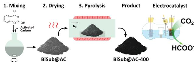
Fig. 1 Synthesis scheme of the BiSub@AC-400 electrocatalyst.
