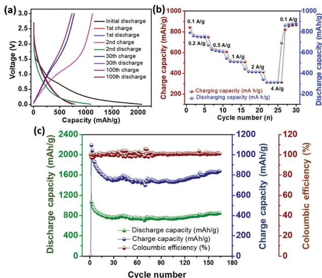
Fig. 3 (a) Discharge–charge voltage profile, (b) rate capability and (c) cycling performance of the electrode containing **3** in the half-cell w. r. t. Li/Li<sup>+</sup>.
