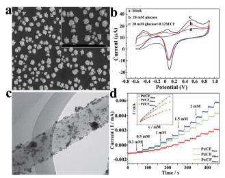
Fig. 8 (a) SEM image of Pt nanoflowers. 77 (b) CV curves of the Pt nanoflower electrode in 0.2 M neutral PBS.<sup>77</sup> (c) TEM image of the Pt nanoparticles on carbon fibers.<sup>80</sup> (d) Amperometric current-time response of Pt/CF in 0.1 M NaOH solution after the successive injection of different concentrations of glucose. 80 Reproduced ref. 77 and 80 with permission from Elsevier B.V., copyright 2011, 2015.
