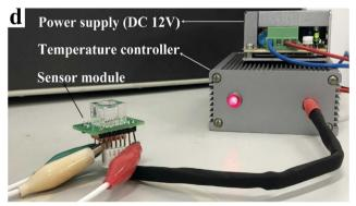
Fig. 16 (a) Optical photograph of the microelectrode module. (b) Typical application of the microelectrode module. (c) Structure of the microelectrode module. (d) Optical photograph of the microelectrode module under working conditions. Reproduced ref. 35 with permission from Elsevier B.V., copyright 2020
