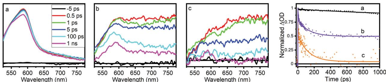
Fig. 3 Optical transient absorption spectra and kinetics (collected at 585 nm) of (a) NH<sub>2</sub>-BDC, (b) NH<sub>2</sub>-MIL-125(Ti,Fe), and (c) NH<sub>2</sub>-MIL-125(Ti).
