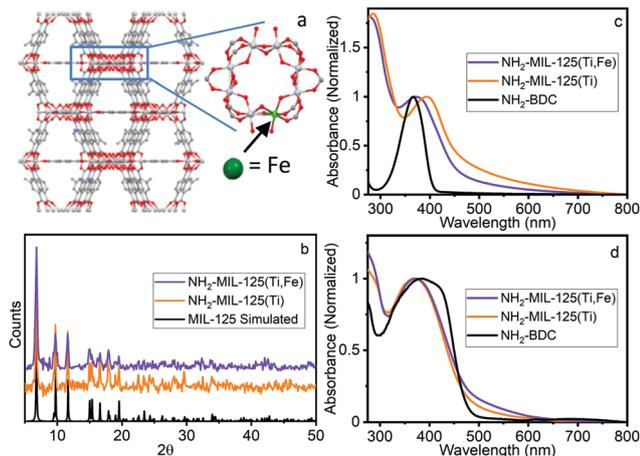
Fig. 1 (a) Proposed structure of  $\text{NH}_2\text{-MIL-125(Ti,Fe)}$ , (b) PXRD, (c) UV-vis absorption and (d) DR spectra of  $\text{NH}_2\text{-BDC}$ ,  $\text{NH}_2\text{-MIL-125(Ti)}$ ,  $\text{NH}_2\text{-MIL-125(Ti,Fe)}$ .
