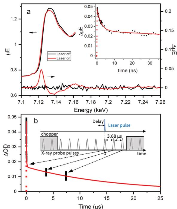
Fig. 4 Fe K-Edge XTA (a) spectra and corresponding difference spectra for  $\text{NH}_2\text{-MIL-125(Ti,Fe)}$ . Inset: Kinetics monitored at 7.123 keV and (b) extended kinetics associated with synchronized and subsequent two X-ray probe pulses. Inset: Schematic representation of XTA timing structure.
