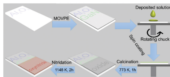
Fig. 3 Schematic illustration of the fabrication procedure for semi-transparent quaternary metal oxynitride thin film photoanode on transparent conductive GaN/Al 2 O 3 substrate.
