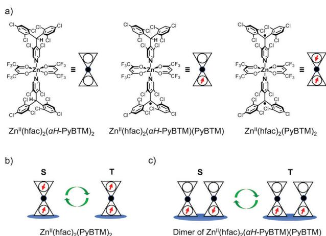
**Fig. 1** (a) Structures of Zn<sup>II</sup>(hfac)<sub>2</sub>( $\alpha$ H-PyBTM)<sub>2</sub>, Zn<sup>II</sup>(hfac)<sub>2</sub>( $\alpha$ H-PyBTM)(PyBTM), and Zn<sup>II</sup>(hfac)<sub>2</sub>(PyBTM)<sub>2</sub>. (b and c) Spin multiplicity changes in (b) Zn<sup>II</sup>(hfac)<sub>2</sub>(PyBTM)<sub>2</sub> and (c) Zn<sup>II</sup>(hfac)<sub>2</sub>( $\alpha$ H-PyBTM)(PyBTM) dimer.
