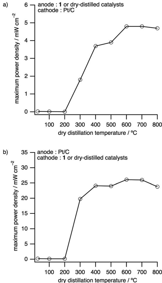
Fig. 5 Maximum power densities of  $\text{H}_2$ - $\text{O}_2$  fuel cells depending on the dry distillation temperature. At the dry distillation temperature of 25 °C, **1** is used as it is as a fuel cell catalyst. (a) Anode: **1** or DDCs. Cathode: Pt/C. (b) Anode: Pt/C. Cathode: **1** or DDCs.
