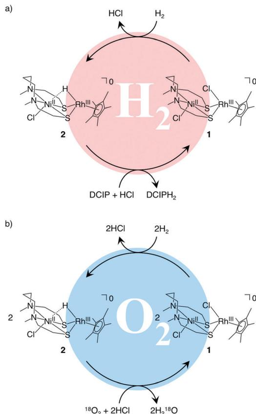
Fig. 2 Proposed catalytic reaction mechanisms for (a)  $\text{H}_2$ -oxidation and (b)  $\text{O}_2$ -reduction with NiRh complexes in water. DCIP: 2,6-dichlorobenzeneindophenol. DCIPH<sub>2</sub>: reduced-form of DCIP.
