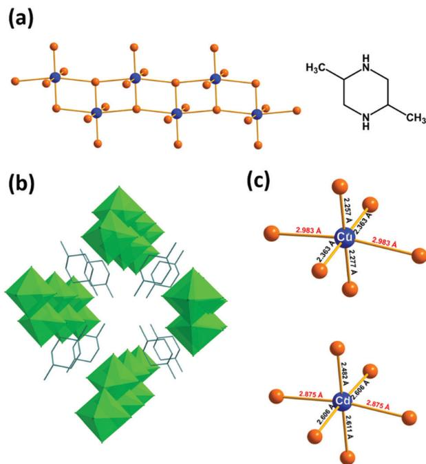
Fig. 1 Representation of (a) the ladder-type structure of copper and cadmium chloride compounds and the *trans*-2,5-dimethylpiperazine (TDMP) molecule, (b) the packing of inorganic ladders and TDMP<sup>2+</sup> cations and (c) the distortion of metal chloride octahedra.
