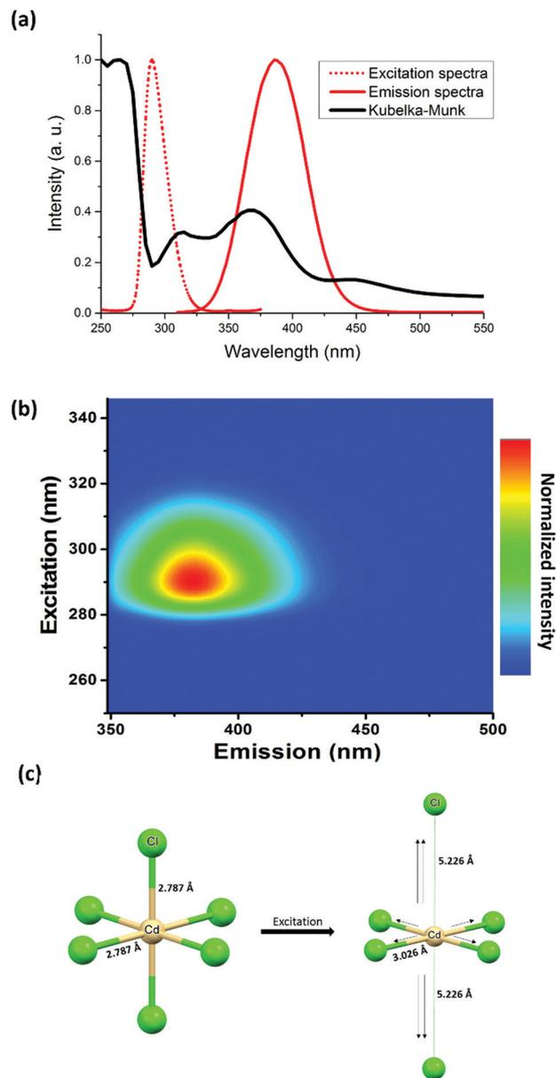
Fig. 2 (a) Absorption, excitation ( $\lambda_{\text{em}} = 385 \text{ nm}$ ), and emission ( $\lambda_{\text{exc}} = 290 \text{ nm}$ ) spectra of (TDMP)CdCl<sub>4</sub>. (b) PL excitation vs. emission mapping of (TDMP)CdCl<sub>4</sub>, and (c) calculated distortion of [CdX<sub>6</sub>]<sup>4-</sup> motifs under excitation.
