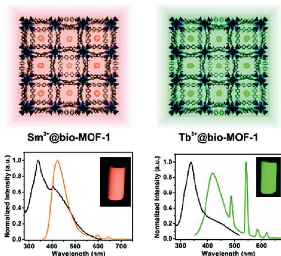
Fig. 7 The encapsulation scheme and luminescence spectra of Sm<sup>3+</sup> (left) and Tb<sup>3+</sup> (right) into bio-MOF-1. Reproduced from ref. 69 with permission from the American Chemical Society, copyright 2011.
