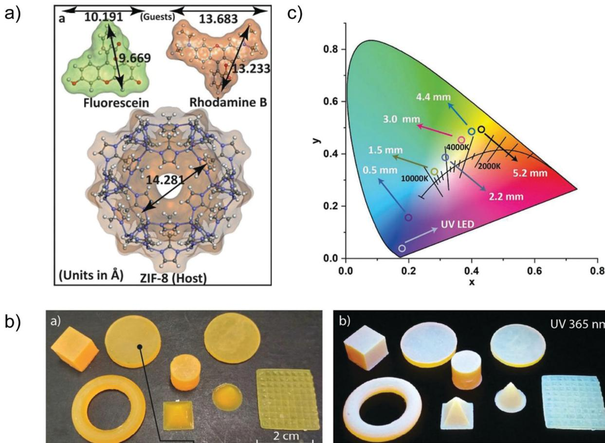
**Fig. 11** (a) Structural dimensions of the two fluorescent guest species FL and RhB, and the host framework of ZIF-8. (b) Various shapes of 3D printed objects constructed from FL + RhB@ZIF-8 dispersed in photopolymer resin, which emit white light under UV irradiation. (c) CIE coordinates corresponding to the cool to warm white light changed by tuning the pellet thickness (given in mm). Reproduced from ref. 72 with permission of John Wiley & Sons, Ltd, copyright 2020.
