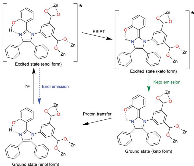
Fig. 6 The ESIP process of hpi2c<sup>2-</sup> linkers in [Zn<sub>6</sub>(hpi)<sub>4</sub>(hpi2c)<sub>4</sub>]. Reproduced from ref. 64 with permission of John Wiley & Sons, Ltd, copyright 2016.
