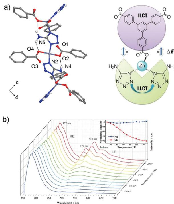
Fig. 3 (a) 1D zigzag chain in [(CH<sub>3</sub>)<sub>2</sub>NH<sub>2</sub>][Zn(btb)<sub>2/3</sub>(atz)] with N-H...O hydrogen bonds (top). The Dexter energy transfer (DET) mechanism in a dual emissive system (down). (b) Emission spectra of [(CH<sub>3</sub>)<sub>2</sub>NH<sub>2</sub>][Zn(btb)<sub>2/3</sub>(atz)] recorded between 10 and 130 K (λ<sub>ex</sub> = 330 nm). Reproduced from ref. 60 with permission of John Wiley & Sons, Ltd, copyright 2016.
