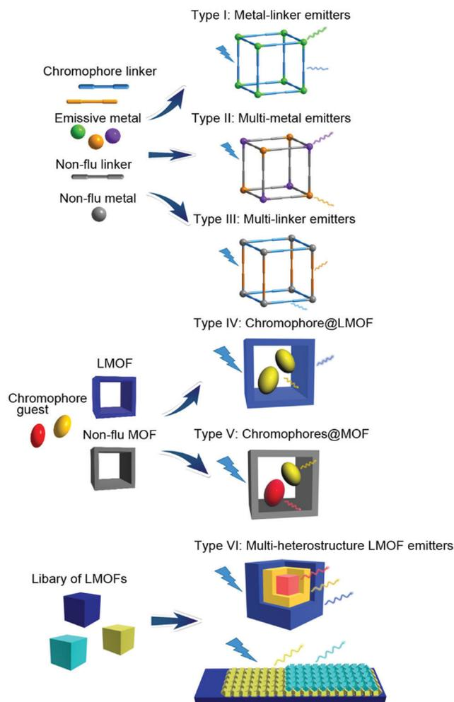
**Scheme 1** Multi-emitter luminescent MOFs (LMOFs) differentiated in a simplified scheme according to the origin of the emission. The scheme also implies that the luminescent metals and linkers can only be doped into a non-luminescent framework. There could also be more than two different luminescent metal, linker or framework types. In the “luminescent framework” building block (LMOF) in Types IV and VI the luminescence can come from either metal or ligand or both.
