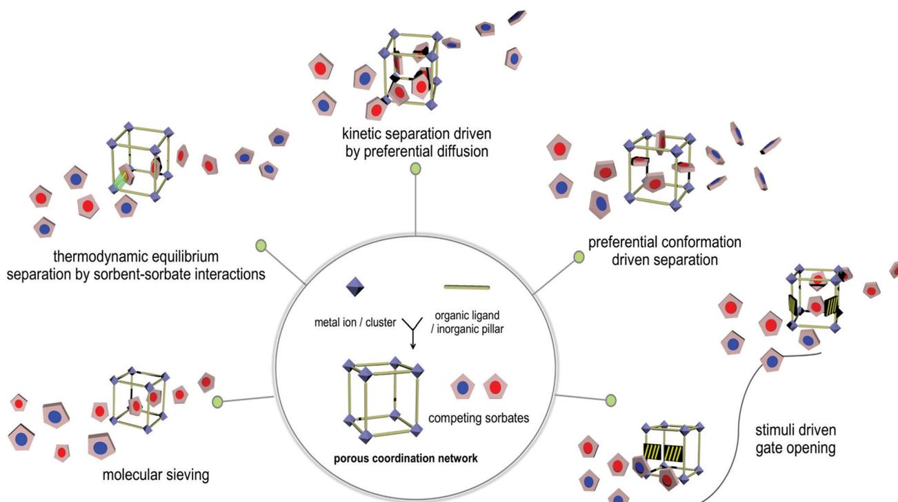
Fig. 5 There are multiple mechanisms for the adsorptive separation of C<sub>2</sub> LHs by PCNs as illustrated clockwise from bottom left: molecular sieving by size/shape exclusion; thermodynamic equilibrium separation; differential diffusivity driven kinetic separation; conformational preference guided separation; stimuli driven network switching based upon separation concomitant with gate opening.
