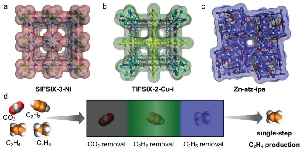
Fig. 15 (a–c) 1D ultramicroporous channels in the **pcu** topology PCN sorbents (a) **SIFSIX-3-Ni**, (b) **TIFSIX-2-Cu-i** and (c) **Zn-atz-ipa**, respectively; (d) SSST to purify C<sub>2</sub>H<sub>4</sub> in one-step from a CO<sub>2</sub>/C<sub>2</sub>H<sub>2</sub>/C<sub>2</sub>H<sub>4</sub>/C<sub>2</sub>H<sub>6</sub> quaternary gas mixture.
