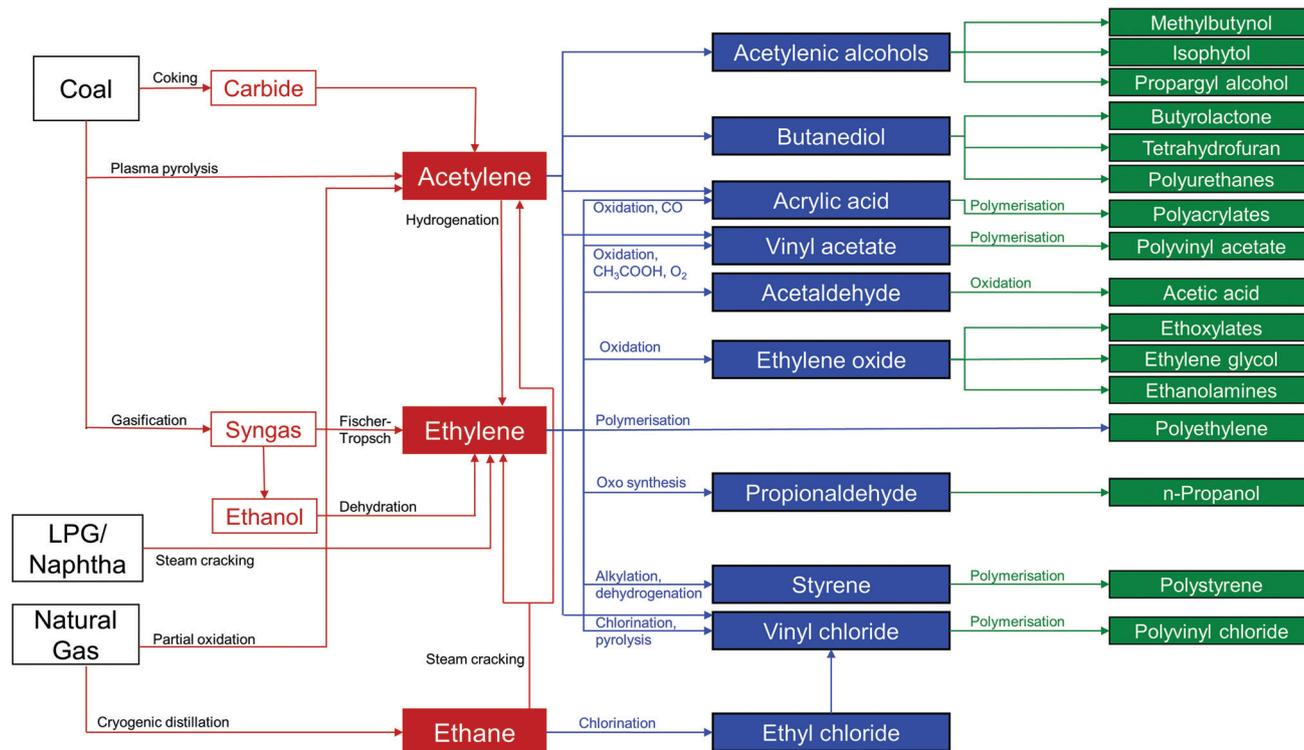
Fig. 1 A schematic of industrial routes for the production of C<sub>2</sub> hydrocarbons and derived products.
