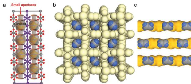
Fig. 10 Schematic illustrations of pore size-controlled uptake of (a)  $\text{C}_2\text{H}_2$  in **SIFSIX-14-Cu-i**;<sup>42</sup> (b and c)  $\text{C}_2\text{H}_4$  in UTSA-280.<sup>57</sup> (Reprinted with permissions from ref. 42 and 57: copyright 2017, Wiley-VCH Verlag GmbH & Co. KGaA, Weinheim; copyright 2018, Springer Nature.)
