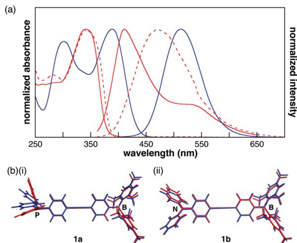
**Fig. 2** (a) UV-vis absorption and emission spectra of **1a** (red) and **1b** (blue) in  $\text{CH}_2\text{Cl}_2$  ( $10^{-5}$  M) (solid line) and the film state (dotted line), (b) optimized structures of (i) **1a** and (ii) **1b** at the  $S_0$  (red) and  $S_1$  (blue) states.
