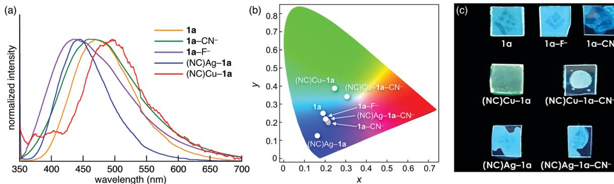
Fig. 5 (a) Changes in the emission spectra, (b) emission colour coordinates in the CIE 1931 chromaticity diagram, and (c) photographs under UV irradiation of **1a** and its complexes with various ion pairs in the film state.
