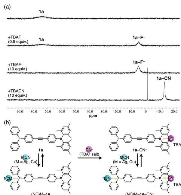
**Fig. 3** (a)  $^{11}\text{B}$  NMR spectra of **1a** (5.5 mM in  $\text{CH}_2\text{Cl}_2$ ) before and after the addition of  $\text{F}^-$  (0.5 and 10 equiv.) and  $\text{CN}^-$  (10 equiv.) as  $\text{TBA}^+$  salts, (b) formation of **1a**- $\text{CN}^-$ ,  $(\text{NC})\text{M}-\mathbf{1a}$ , and  $(\text{NC})\text{M}-\mathbf{1a}-\text{CN}^-$  complexes ( $M = \text{Ag}, \text{Cu}$ ).
