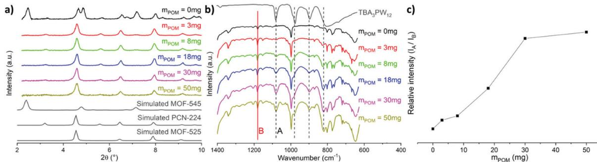
Fig. 3 Impact of a stepwise increase of the amount of  $PW_{12}$  in the synthesis medium of  $PW_{12}@Zr_6-TCCP-Fe-120$  on its (a) PXRD and (b) IR spectra where black dashed lines indicate bands characteristic of  $PW_{12}$  while the red line indicates a band of the MOF host. (c) Evolution of the ratio between the intensities of the A and B bands (see text).
