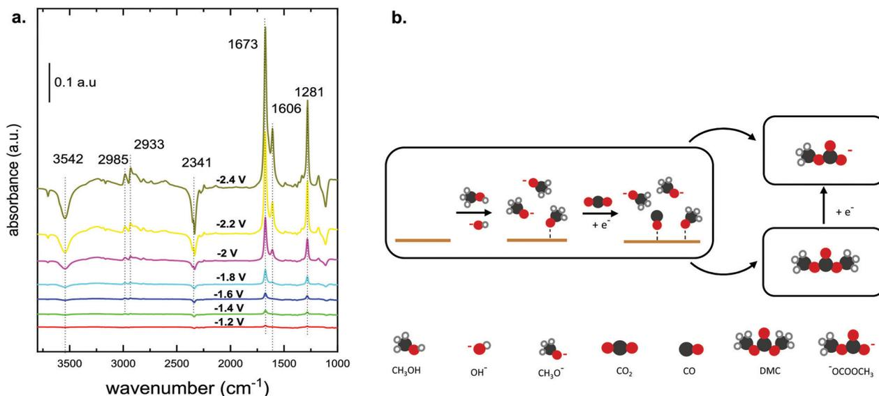
Fig. 3 (a) FTIR spectrum of CO<sub>2</sub> reduction in CH<sub>3</sub>OH on a Cu electrode at potentials between -1.2 and -2.4 V vs. Ag/AgCl.<sup>10</sup> (Reprinted with permission from American Chemical Society. Copyright © 2019, American Chemical Society.) (b) Proposed reaction mechanism that involves the electrochemical reduction of CO<sub>2</sub> to CO with a simultaneous activation of CH<sub>3</sub>OH. Scheme adapted from ref. 10.
