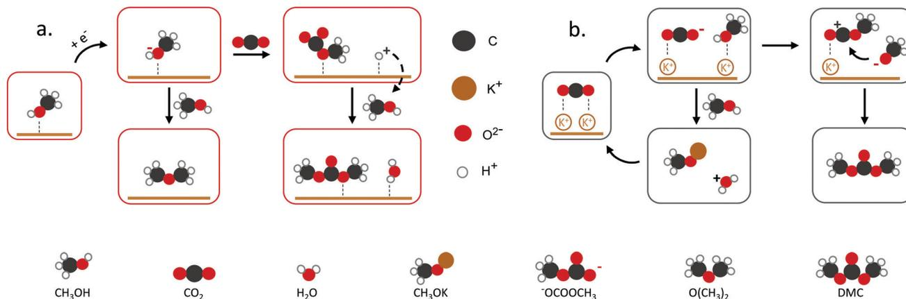
Fig. 2 Proposed mechanisms towards DMC. (a) DMC formation through methoxy and CO<sub>2</sub>, (b) K<sup>+</sup> interaction with CO<sub>2</sub> to DMC. Figures adapted from ref. 25 and 33.
