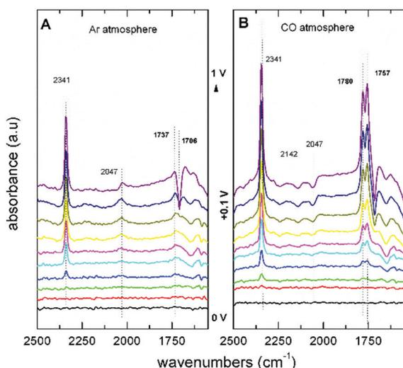
Fig. 6 FTIR spectra of an Au electrode in 0.1 M  $LiClO_4$  in  $CH_3OH$  with 0.1 M PhOH saturated with (A) Ar and (B)  $CO$ .<sup>55</sup> Reprinted with permission from American Chemical Society. Copyright©2019, American Chemical Society.
