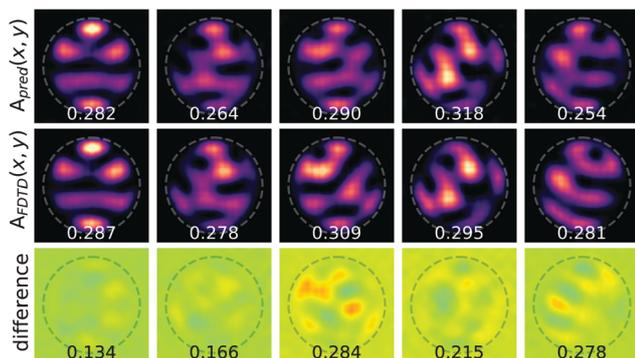
Fig. 2 Randomly chosen examples of the MLP-predicted profile  $A_{pred}$ , the corresponding true profile  $A_{FDTD}$ , and the difference between the two profiles (difference). The integrated absorption ( $\lambda = 600$  nm) for each profile is included at the bottom of each panel. The  $\sigma_{pp}$  metric for each pair is included at the bottom of the difference panel.
