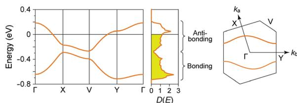
Fig. 15 Electronic band dispersions, densities of states ( $D(E)$  in states per electronvolt per spin), and Fermi surfaces of  $(\text{TMTTF})_2\text{PF}_6$ , calculated on the basis of the extended Hückel method with the tight-binding approximation using crystallographic data at room temperature. The energy is provided relative to the Fermi energy. Note that the electron–electron correlation is not considered in this calculation.
