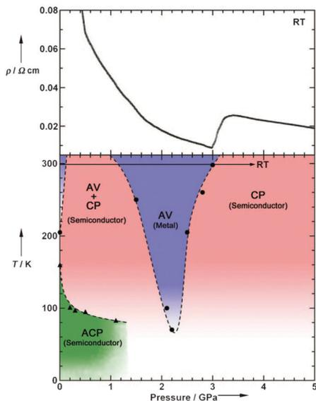
Fig. 8 (Upper) Pressure dependence of room-temperature resistivity ( $\rho$ ) and (lower) electronic  $T$ - $P$  phase diagram of  $\text{Pt}_2(\text{EtCS}_2)_4\text{I}$ , where a panel presented in the original paper<sup>32</sup> was omitted. Adapted with permission from ref. 32. Copyright 2009 Wiley-VCH.
