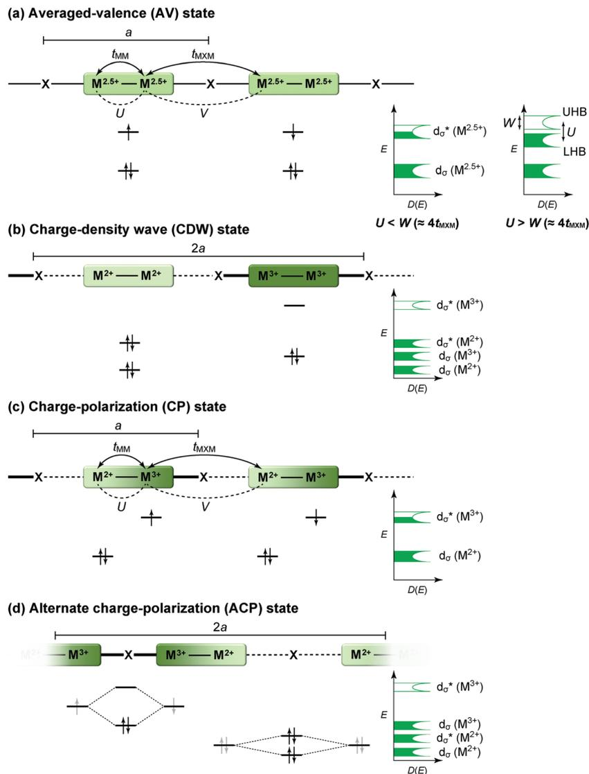
Fig. 3 Schematic electronic structures of the typical states in MMX-chain complexes: (a) averaged-valence (AV) state, (b) charge-density wave (CDW) state, (c) charge-polarization (CP) state, and (d) alternate charge-polarization (ACP) state ( $a$ : periodicity of an  $-M-M-I-$  unit,  $t_{MM}$ : transfer energy within an MM subunit,  $t_{MXM}$ : transfer energy between the subunits,  $V$ : inter-site Coulomb repulsion energy).<sup>18</sup>
