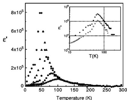
Fig. 19 Temperature dependence of the real part of the dielectric permittivity ( $\epsilon'$ ) of  $(\text{TMTTF})_2\text{PF}_6$  at different frequencies: 1 kHz ( $\oplus$ ), 10 kHz ( $\blacktriangle$ ), 100 kHz ( $\bullet$ ), 1 MHz ( $\blacksquare$ ), and 5 MHz ( $\blacklozenge$ ). Inset shows the difference between the  $\epsilon'$  of the salt obtained from different batches (100 kHz). Adapted with permission from ref. 92. Copyright 2000 American Physical Society.
