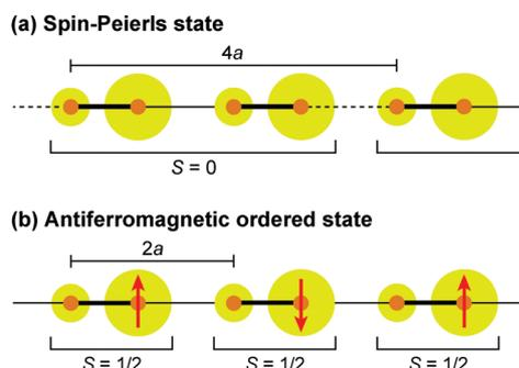
Fig. 20 Schematic electronic structures of (a) spin-Peierls state in  $(\text{TMTTF})_2\text{PF}_6$  and  $(\text{TMTTF})_2\text{AsF}_6$  and (b) antiferromagnetic ordered state in  $(\text{TMTTF})_2\text{SbF}_6$ .<sup>94</sup> Red arrows indicate a magnetically ordered spin, and other specifications are the same as those used in Fig. 17.
