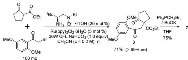
Scheme 6 Catalytic asymmetric construction of the quaternary stereocenter.
