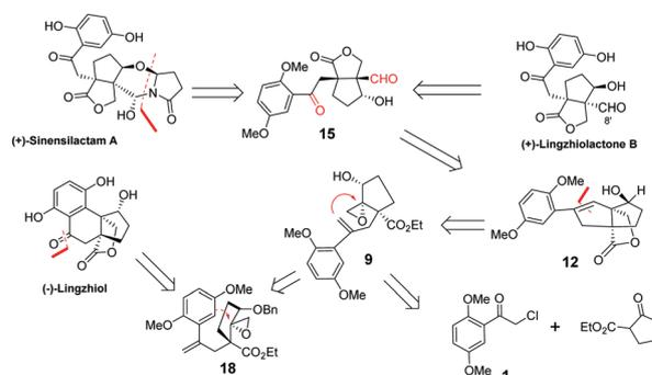
Fig. 1 Structures of several meroterpenoids and retrosynthetic analysis.
