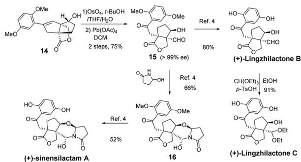
Scheme 3 Completion of the synthesis of (+)-sinensilactam A.
