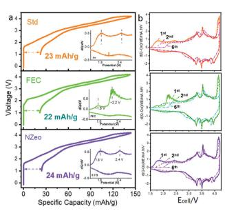
Fig. 1 The electrochemical performance of  $Na_aMO_2/C$  cells using different electrolyte with additives. (a) Initial voltage–capacity curve of the cell and (b) differential capacity plot of the full cells. Differential capacity plots of the  $Na_aMO_2/C$  cells. Different line styles represent the 1st, 2nd and 6th cycle.
