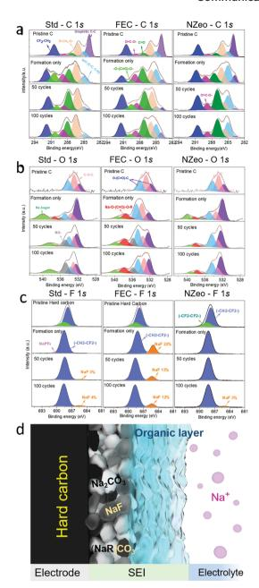
Fig. 3 The XPS spectra of pristine hard carbon electrodes and those electrodes after formation, after 50 cycles and after 100 cycles by using Std, FEC and NZeo electrolytes. (a) The C 1s spectra of hard carbon electrodes; (b) O 1s spectra of the hard carbon e electrodes; (c) F 1s spectra of the hard carbon electrodes. (d) Schematic illustration of the SEI layer.
