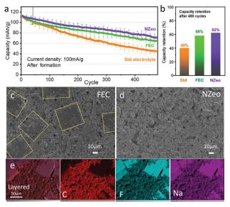
Fig. 2 The capacity performance of the full cell using different additives. (a) Long cycle performance and (b) capacity retention during long cycling at 100 mA  $\rm g^{-1}$  after 5 formation cycles at 10 mA  $\rm g^{-1}$ . SEM images of the nonplating regions of the anode coating for FEC (c) and NZeo (d) electrolytes after 480 cycles; mapping images of the flakes pattern observed on the negative electrode surface with the presence of FEC (e).
