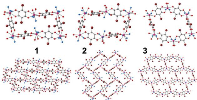
Fig. 1 (up) Cavities in compounds **1–3** (down). The disposition of the cavities in the layers in **1–3**. Only the O atoms of the coordinated solvent molecules are shown for clarity. Colour code: C = grey, Br = brown, O (anilato) = red, O (solvent) = blue, Dy = pink.
