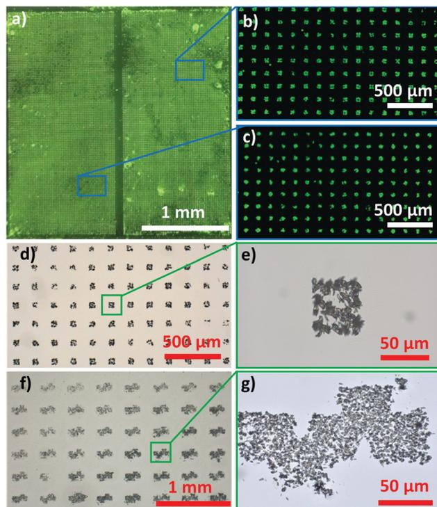
**Fig. 3** (a) Photograph of the Tb-MOF pattern on glass under UV light (254 nm); (b and c) magnified patterned regions under UV light (254 nm); (d and e) optical microscopy image of the Tb-MOF in a square pattern and its magnification; (f and g) optical microscopy image of the Tb-MOF in a TU Graz Logo pattern and its magnification. All these Tb-MOF patterns were obtained via the biomimetic replication of palmitic acid patterns.
