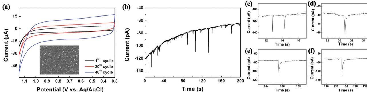
Fig. 1 (a) Electropolymerization of EDOT by cyclic voltammetry (0.1 M EDOT, 0.2 M TBAP in DCM at  $50 \text{ mV s}^{-1}$  scan rate; inset displays resultant film by SEM). (b) Chronoamperogram exhibiting collision signals of 200 nm droplets onto a  $10 \mu\text{m}$  carbon electrode, with each oxidation spike leading to a synthesized PEDOT NP. (c)–(f) Typical single droplet electrolysis signals. See also Fig. S2 and S3 (ESI†).
