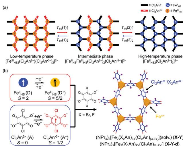
**Scheme 1** Schematic representations of the investigated tetraoxolene-bridged Fe honeycomb layers. (a) The variations of charge-ordered states in **0** and **0-d**, where for **0**,  $T_{1/2(1)}$  was  $T_{1/2a}$  (i.e., there was no high-temperature phase for **0**), and for **0-d**,  $T_{1/2(1)}$  and  $T_{1/2(2)}$  correspond to  $T_{1/2b}$  and  $T_{1/2c}$ , respectively. (b) Schematic route for the syntheses of site-doped solid solution compounds in this work.
