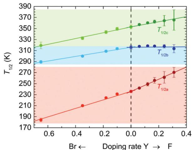
Fig. 4 Variations of the  $T_{1/2}$  value of TDETs for the site-doped rate  $Y$  in the solid solution series of  $X-Y$  and  $X-Y-d$ , whereas the basis of  $Y = 0$  corresponded to  $0$  and  $0-d$ . The left and right scales represent  $Br-Y/Br-Y-d$  and  $F-Y/F-Y-d$ , respectively. The solid lines are least-square linear fitting lines for the respective series.
