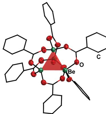
Fig. 4 Molecular structure of  $[(\text{Be}_4\text{O})(\text{PhCO}_2)_6]$  (**7**) in the solid state.<sup>50</sup> The tetrahedron of the central  $[\text{Be}_4\text{O}]^{6+}$  core is highlighted in red. Ellipsoids are depicted at 70% probability at 143 K. Carbon atoms are depicted as wire frame and hydrogen atoms are omitted for clarity.
