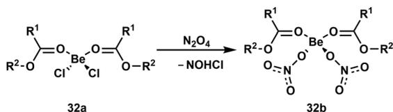
Scheme 6 Displacement of chlorido by nitrate ligands in beryllium esters.  $\text{R}^1 = \text{H, Me}$ ;  $\text{R}^2 = \text{Me, Et, } {}^i\text{Pr}$ .<sup>92</sup>
