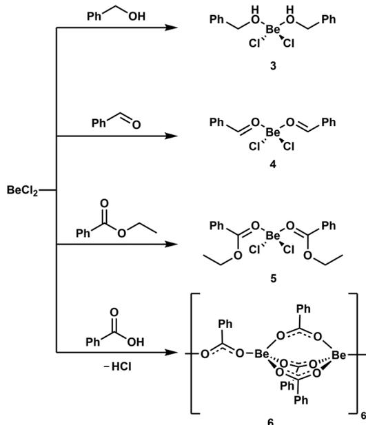
Scheme 2 Reaction of  $\text{BeCl}_2$  with benzyl alcohol, benzaldehyde, ethyl benzoate and benzoic acid.<sup>49</sup>
