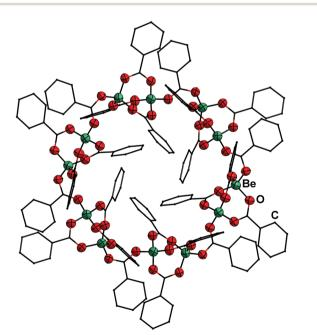
Fig. 3 Molecular structure of [Be(PhCO $_2$ ) $_2$ ] $_{12}$  (6) in the solid state. Ellipsoids are depicted at 70% probability at 100 K. Carbon atoms are depicted as wire frame and hydrogen atoms are omitted for clarity.<sup>49</sup>
