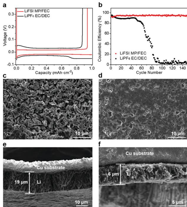
**Fig. 1** Li metal performance in the selected electrolytes at room temperature. (a) Li plating/stripping curves and (b) long-term cycling performance of Li||Cu cells in LiFSI MP/FEC, and LiPF<sub>6</sub> EC/DEC at 0.5 mA cm<sup>-2</sup>; top (c and d) and cross-section (e and f) views of the SEM images of Li deposits obtained in LiPF<sub>6</sub> EC/DEC (c and e) and LiFSI MP/FEC (d and f) at 1 mA h cm<sup>-2</sup> and 0.5 mA cm<sup>-2</sup>.
