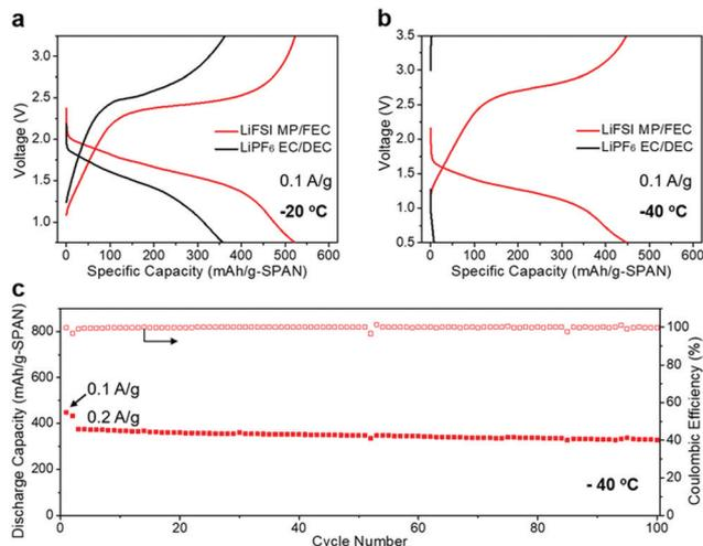
**Fig. 3** Li||SPAN half cell performance at ultra-low temperatures. Voltage curves of Li||SPAN cells at (a)  $-20\text{ }^{\circ}\text{C}$  and (b)  $-40\text{ }^{\circ}\text{C}$  with a current density of  $0.1\text{ A g}^{-1}$  in each electrolyte; (c) long-term cycling performance of Li||SPAN half cells charging and discharging at  $-40\text{ }^{\circ}\text{C}$  in LiFSI MP/FEC.
