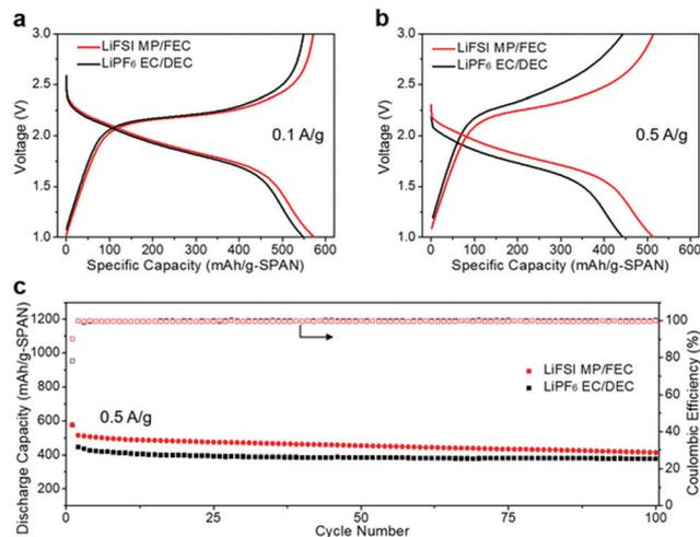
**Fig. 2** Li||SPAN half-cell performance in different electrolytes at room temperature. Voltage curves at (a) 0.1 A g<sup>-1</sup> and (b) 0.5 A g<sup>-1</sup>; (c) long-term cycling performance at 0.5 A g<sup>-1</sup>.
