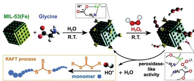
Fig. 10 Proposed mechanisms for the formation of Gly/MIL-53(Fe) and the initiation of RAFT polymerization by hydroxyl radicals. Reproduced with permission.<sup>51</sup> Copyright 2018 The Royal Society of Chemistry.
