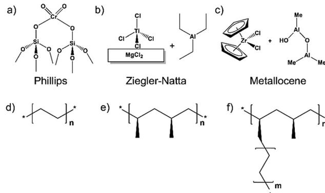
**Fig. 1** Structures of (a) Phillips catalyst (proposed), (b) Ziegler–Natta supported catalyst, (c) example metallocene catalyst, (d) linear polyethylene, (e) isotactic polypropylene, and (f) example specialty copolymer of propylene and ethylene.
