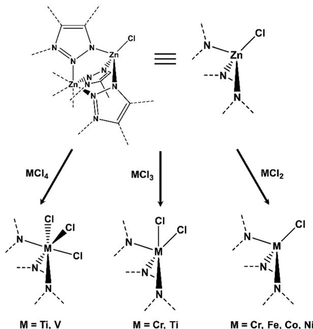
Fig. 7 Scope of published cation exchange in MFU-4l used for polymerization catalysis.<sup>42-45</sup>
