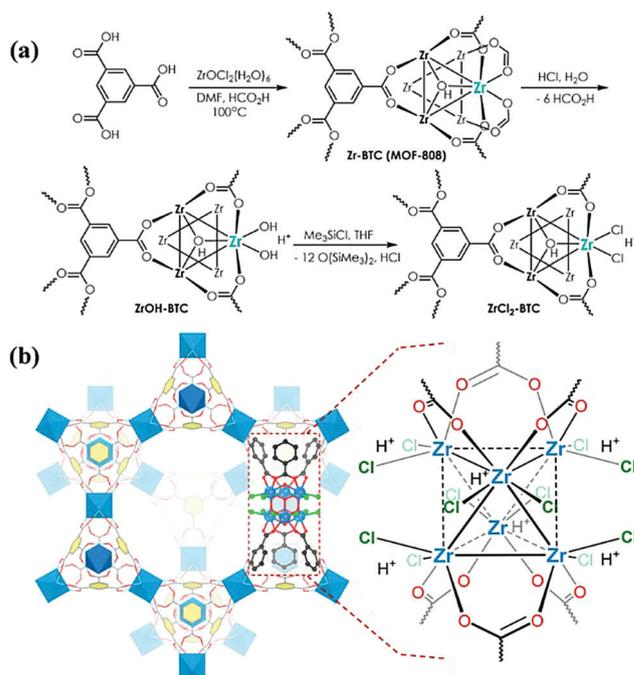
Fig. 6 (a)  $ZrCl_2$ -BTC synthetic scheme beginning with synthesis of Zr-BTC (MOF-808) and (b) proposed structure of  $ZrCl_2$ -BTC. Reprinted with permission.<sup>41</sup> Copyright 2017 American Chemical Society.
