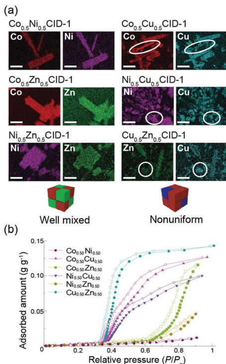
Fig. 4 (a) SEM-EDX maps for  $M_{1.0.5}M_{2.0.5}CID-1$ . White circles indicate nonuniform areas. Scale bars: 30  $\mu\text{m}$ . (b) Water-sorption isotherms of  $M_{1.0.5}M_{2.0.5}CID-1$  at 298 K. Filled and open symbols correspond to adsorption and desorption, respectively.
