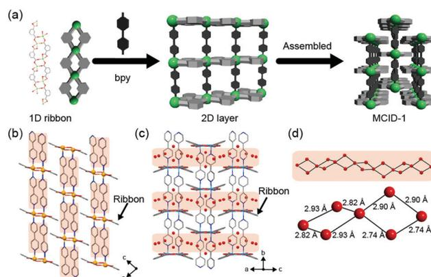
**Fig. 1** (a) MCID-1 assembly process. Crystal structures of (b) CoCID-1, (c) CuCID-1·H<sub>2</sub>O, and (d) CuCID-1. The pale-red highlighted regions in (b) and (c) represent pore spaces. The pale-red highlighted region in (c) represents the water chain structure in the 1D channel. Orange, gray, blue, and red represent Co, C, N, and O, respectively. H atoms are omitted for clarity.
