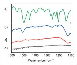
Fig. 2 ATR-FTIR spectra of (a) Sudan I, (b) TiO<sub>2</sub>-1, (c) TiO<sub>2</sub>-APSil, and (d) TiO<sub>2</sub>-Bare. Spectra (b) through (d) were rescaled, to the same degree, in order to more easily compare their features with the powder sample, (a).
