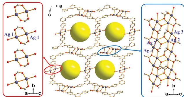
Fig. 1 The framework structure of **AgBTB** with an array of finite  $[\text{Ag}_2(\text{COO})_2]$  dinuclear clusters and an infinite  $[\text{Ag}_4(\text{COO})_4]_n$  1D ribbon.
