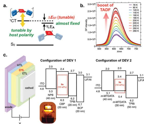
Fig. 6 (a) A schematic illustration of energy diagrams of D–A–D compounds **9**, (b) temperature-dependency of the PL spectra of **9d** in CBP host, and (c) configurations of OLED devices fabricated with **9d**. The inset photograph shows the OLED device (DEV 1). Adapted from ref. 21. Copyright 2016 Wiley-VCH Verlag GmbH.
