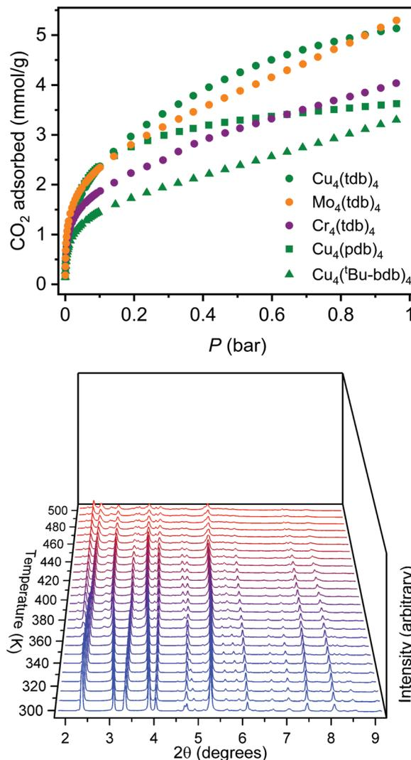
Fig. 3 (Top)  $CO_2$  adsorption in  $M_4(L)_4$  cages at 195 K. (Bottom) PXRD patterns as a function of temperature for  $Cu_4(tdb)_4$  spanning the temperature range of 300–550 K. During this activation, the cage remains moderately crystalline while undergoing significant structural rearrangement.
