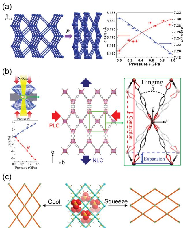
Fig. 16 Scheme of the wine-rack structural changes under hydrostatic pressure that exhibit NLC. (a)  $[\text{NH}_4][\text{Zn}(\text{HCOO})_3]$ . (b)  $\text{InH}(\text{BDC})_2$ . (c)  $[\text{Ag}(\text{ethylenediamine})]\text{NO}_3$ . Partly taken from ref. 111, 113, and 116 with permission.
