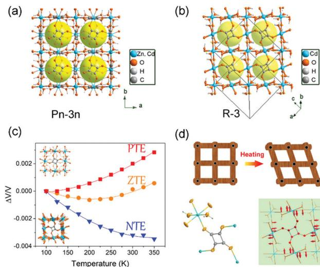
Fig. 11 Crystal structure of the cubic phase (a) and trigonal phase (b) of  $\text{MC}_4\text{O}_4 \cdot 2\text{H}_2\text{O}$  ( $M = \text{Zn}, \text{Cd}$ ). (c) Temperature-dependent relative volume changes of the three compounds. (d) Scheme of the wine-rack distortion of the framework in the trigonal phase  $\text{Cd\_sq\_R}$  and illustration of the transverse vibration of the squarate ligand. Reprinted with permission from ref. 93.
