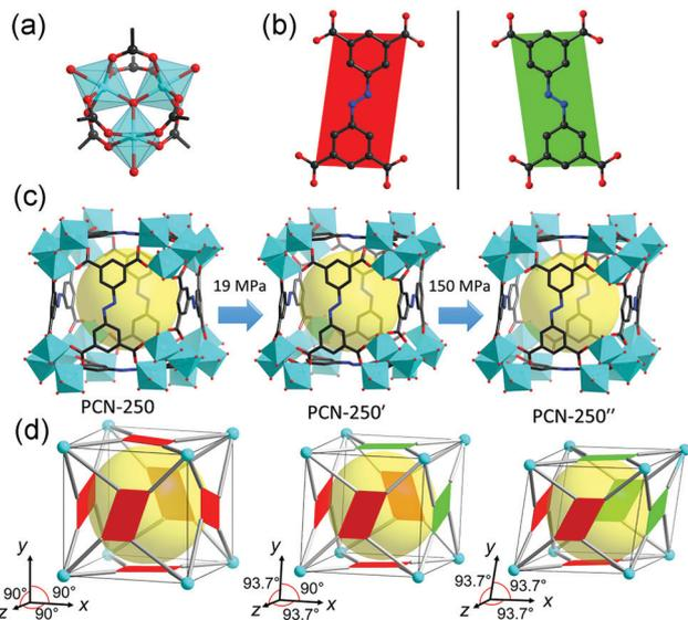
**Fig. 20** (a) Structure of the  $\text{Fe}_3$ -oxo cluster. (b) ABTC ligand with two different kinds of configurations. (c) Crystal structure of PCN-250 at different pressures. (d) Scheme of the pressure induced structural transformation including the inclination of unit cell and flipping of ligands. Reprinted with permission from ref. 126.
