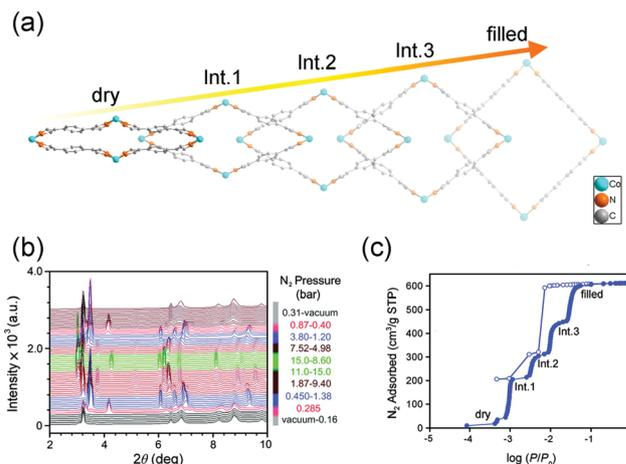
Fig. 3 (a) Scheme of the continuous breathing behavior of the  $\text{Co}(\text{BDP})$  during  $\text{N}_2$  adsorption. (b) *In situ* X-ray powder diffraction patterns of  $\text{Co}(\text{BDP})$  measured under different gas pressure at 100 K. (c)  $\text{N}_2$  adsorption isotherm measured at 77 K, indicating the five pressure-dependent phases. Filled and empty symbols represent adsorption and desorption, respectively. Modified and reprinted with permission from ref. 58.
