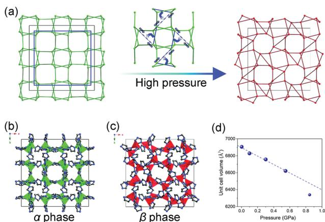
**Fig. 18** (a) Scheme of the framework change under high pressure. Crystal structure of ZIF-zni in  $\alpha$  phase (b) and  $\beta$  phase (c). (d) Unit cell volume of ZIF-zni at different temperatures. Partly taken from ref. 123 with permission.
