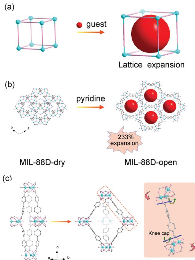
**Fig. 1** (a) Scheme of the guest insertion induced lattice expansion. (b) Crystal structure of the MIL-88D before and after pyridine loading. (c) The cage structure in MIL-88D before (left) and after (middle) guest loading. Right: Illustration of the framework displacements during swelling, which occur around the knee cap O–O axis (blue lines and green arrows). This allows the rotation around this axis of the whole trimeric units (red arrows). Partly taken from ref. 19 with permission.
