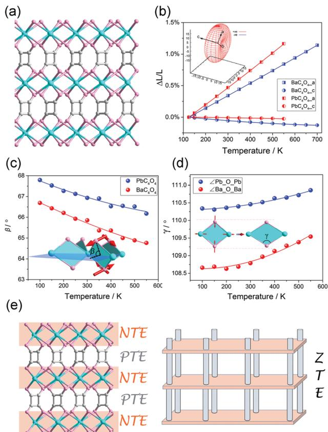
**Fig. 9** (a) Crystal structure of pillar-layered  $MC_4O_4$  ( $M = Ba, Pb$ ). (b) Lattice parameter changes of the  $MC_4O_4$  ( $M = Ba, Pb$ ) obtained from Le bail fitting. (c) Illustration of the out-plane rotation and geometric deformation of a rhombic  $Pb_2O_2$  (or  $Ba_2O_2$ ) plane. (d) Scheme of the mechanism of 1D ZTE which concerns of the NTE in the inorganic layers and PTE of the organic pillar. Reprinted with permission from ref. 84.
