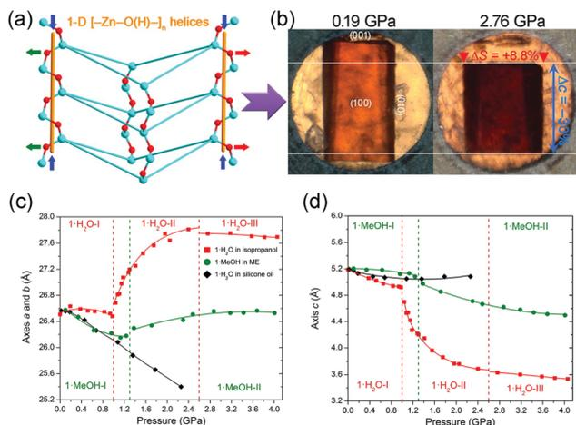
**Fig. 17** (a) A perspective view of the quadrangular rings connected by the  $[-\text{Zn}-\text{O}(\text{H})-]_n$  helices to form a column along the  $c$  axis. (b) Photograph of a single crystal of  $[\text{Zn}(\text{L})_2(\text{OH})_2]\cdot\text{H}_2\text{O}$  compressed in isopropanol in the diamond-anvil cell (DAC) chamber. Lattice parameter changes along  $a$  axis (c) and  $c$  axis (d). Reprinted with permission from ref. 117.
