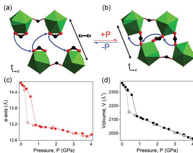
**Fig. 19** Partial crystal structure changes of the  $[\text{tmenH}_2][\text{Er}(\text{HCOO})_4]_2$  before (a) and after (b) compression. Lattice parameter changes of  $a$  (c) and volume (d). The data collected with increasing and decreasing pressure are plotted with filled and empty spheres, respectively. Reprinted with permission from ref. 124.
