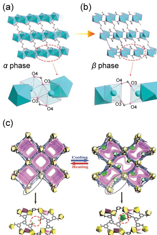
Fig. 13 Illustration of the structural changes of  $[\text{Yb}_2(\text{C}_4\text{H}_4\text{O}_4)_3]$  at low (a) and high (b) temperatures. Top: The overview of the framework. Bottom: Local SBU changes. (c) Scheme of the temperature induced structural changes. Top: The overview of the 3D framework. Bottom: The local enlarged view of the structural difference. Partly taken from ref. 99 and 100 with permission.
