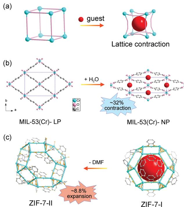
**Fig. 2** (a) Scheme of the guest insertion induced lattice contraction. Illustration of the crystal structure changes of MIL-53 (b) and ZIF-7 (c) during the guest insertion and desolvation. Partly taken from ref. 15 and 55 with permission.
