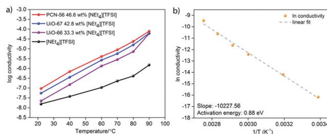
**Fig. 4** (a) Temperature dependence of conductivity of  $[\text{NEt}_4][\text{TFSI}]$  and three  $[\text{NEt}_4][\text{TFSI}]$ -MOF composites, and (b) Arrhenius plot for the conductivity of the PCN-56- $[\text{NEt}_4][\text{TFSI}]$  composite with 46.6 mass%  $[\text{NEt}_4][\text{TFSI}]$ .
