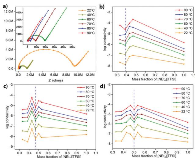
**Fig. 3** (a) Nyquist plots for the UiO-67 composite with 42.8 mass%  $[\text{NEt}_4][\text{TFSI}]$  at temperatures from 22 °C to 90 °C. Plots of the  $\log(\text{conductivity})$  versus the mass fraction of  $[\text{NEt}_4][\text{TFSI}]$  in composites with (b) UiO-66, (c) UiO-67, and (d) PCN-56. The dashed blue line represents the maximum salt loading that can be achieved experimentally for each MOF.
