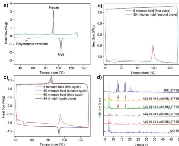
Fig. 2 DSC traces of (a) neat [NEt<sub>4</sub>][TFSI], (b) 38.4% [NEt<sub>4</sub>][TFSI] and 61.6% UiO-67 by mass, and (c) 50.0% [NEt<sub>4</sub>][TFSI] and 50.0% UiO-67 by mass. (d) PXRD pattern of [NEt<sub>4</sub>][TFSI], UiO-66, and various mixtures of the two after heating at 130 °C for 30 min and cooling to room temperature.
