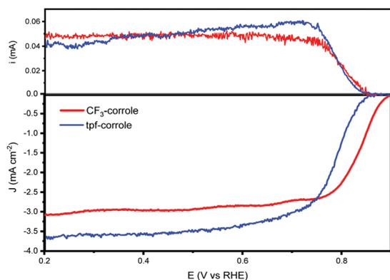
Fig. 2 RRDE of CF<sub>3</sub>-corrole and tpf-corrole in 0.1 M KOH @ 900 rpm.
