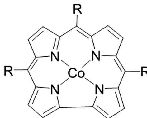
Fig. 1 The structure of Cobalt (III) corrole. CF<sub>3</sub>-corrole R = CF<sub>3</sub> (trifluoromethyl), tpf-corrole R = C<sub>6</sub>F<sub>5</sub> (tris-pentafluoro phenyl).
