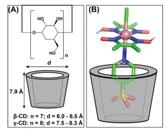
Fig. 15 (A) The basic structure of  $\beta$ - and  $\gamma$ -cyclodextrins (cyclic oligosaccharides of glucose) and their corresponding sizes. (B) The possible interaction between the sulfonate group from cobaloxime [Co(dmgH)2-(pyridine-4-sulfonate)Cl] and the  $\gamma$ -cyclodextrin. These figures were redrawn from ref. 122.
