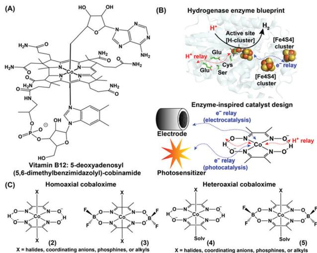
**Fig. 1** (A) Chemical structures of the vitamin B12 core (cobinamide). (B) Inclusion of the  $\text{H}^+$  relay and electron channel around the metal active site in the hydrogenase enzyme (PDB: 1HFE) and synthetic cobaloxime. The electron for the synthetic cobaloxime is transported from the electrode (electrocatalysis) or excited photosensitizer (photocatalysis). (C) Comparative structures of homo- and hetero-axial cobaloximes.
