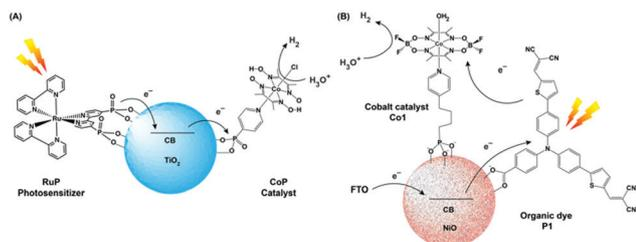
Fig. 9 (A) Schematic representation of photocatalytic  $\text{H}_2$  production  $\text{TiO}_2$  NPs containing a covalently attached cobalt catalyst (CoP) and a ruthenium photosensitizer (RuP). (B) Representative figure of the photocathode containing organic dye P1 and cobaloxime catalyst Co1 on the NiO surface. The figures are redrawn from ref. 78 and 79 respectively.
