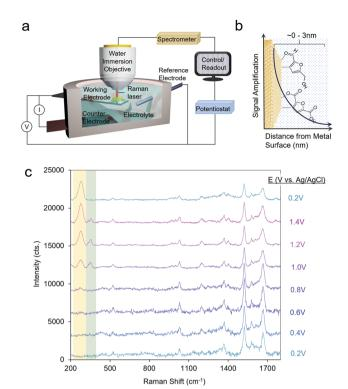
**Fig. 2** A typical reaction cell for *operando* SERS measurements (a), which investigate species precisely at the catalyst–electrolyte interface (b). SERS spectra of HMF oxidation on Au. Reprinted from ref. 28 (N. Heidary and N. Kornienko, *Chem. Commun.*, 2019, **55**, 11996–11999). Copyright 2019 Royal Society of Chemistry.
