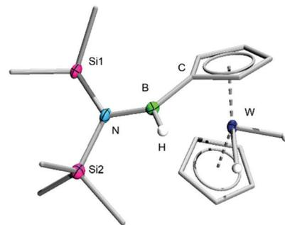
Fig. 1 Crystallographically-determined solid-state structure of **3**. Atomic displacement ellipsoids depicted at 50% probability level. Carbon ellipsoids and most hydrogen atoms are omitted for clarity.
