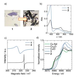
Fig. 3 (a) Colour change from  $\bf 1$  to  $\bf 2$  achieved by chemical doping. (b) Solid-state UV-Vis-NIR diffuse reflectance spectra of  $\bf 1$  (blue) and  $\bf 2$  (black). (c) ESR spectra of  $\bf 1$  (blue) and  $\bf 2$  (black). (d) XANES spectra of the Cu K-edge for  $\bf 1$  (blue),  $\bf 2$  (black), Cu foil (green), Cu<sub>2</sub>O (black dashed line), and CuO (blue dashed line).
