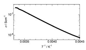
Fig. 5 Temperature dependence of the electrical conductivity  $(\sigma)$  of 2 measured by using a two-probe method on a pellet sample.
