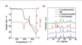
**Fig. 2** (a) TGA and DTA trace of **1**. (b) PXRD patterns of **1d** (red) and **1** (simulated from the crystal structure: purple, experimental: blue, after soaking **1d** in chloroform for a day: green).
