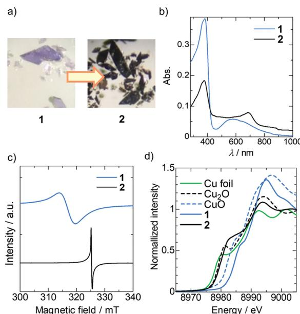
**Fig. 3** (a) Colour change from **1** to **2** achieved by chemical doping. (b) Solid-state UV-Vis-NIR diffuse reflectance spectra of **1** (blue) and **2** (black). (c) ESR spectra of **1** (blue) and **2** (black). (d) XANES spectra of the Cu K-edge for **1** (blue), **2** (black), Cu foil (green),  $\text{Cu}_2\text{O}$  (black dashed line), and CuO (blue dashed line).
