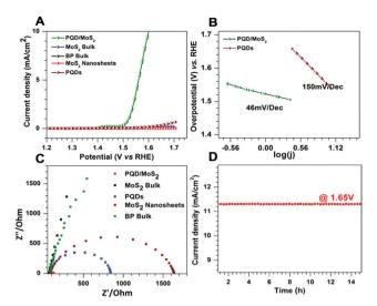
**Fig. 2** (A) LSVs acquired for determining the OER activities of various samples in 0.1 M KOH solutions at 1600 rpm. (B) Tafel plots of PQD/MoS<sub>2</sub> and PQDs measured from the corresponding LSVs in (A). (C) Impedance spectra of PQD/MoS<sub>2</sub> and of the other indicated samples. (D) Chrono-amperometric response of PQD/MoS<sub>2</sub>, indicating their long-term durability.
