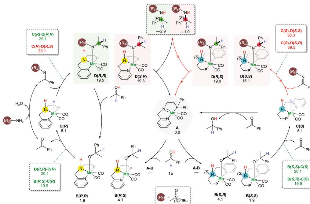
**Scheme 2** Proposed reaction mechanism for the stereoselective manganese catalysed hydrogen autotransfer amination of *rac*-alcohols. Free reaction and activation energies (at 140 °C) are shown in kcal mol<sup>-1</sup> at the M06/TZVP level using toluene as a solvent.
