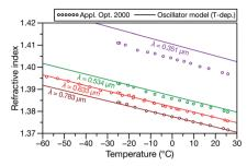
Fig. 5 RI measurements at four different wavelengths for an aqueous solution containg  $H_2SO_4$  and  $HNO_3$  ( $\phi_{H_2SO_4}=0.1741$  and  $\phi_{HNO_3}=0.1741$ ) from ref. 32 compared to the temperature-dependent effective oscillator model ( $\kappa=-0.0015~\text{K}^{-1}$ ).
